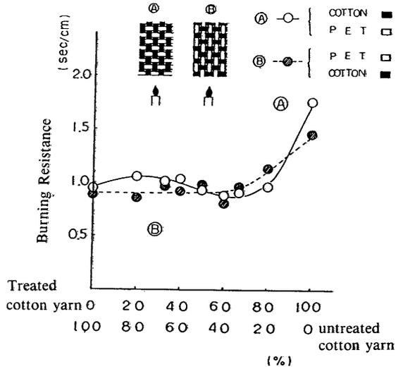
Fig. 2 Effect of the ratio of the THPC treated cotton yarn and untreated one on the burning resistance for the union cloth (cotton /polyester = 50/50)
