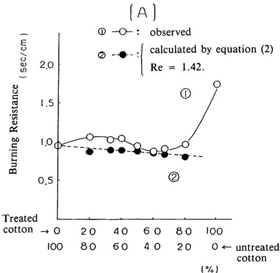
Fig 4 (A) Observed (—○—) and calculated (---●---) burning resistance for the union cloth (treated cotton yarn and untreated one: untreated polyester yarn = 50:50)
