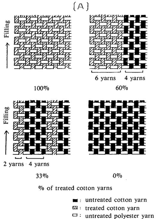
Fig. 1 (A) Diagram of the ratio of treated/untreated cotton yarn
