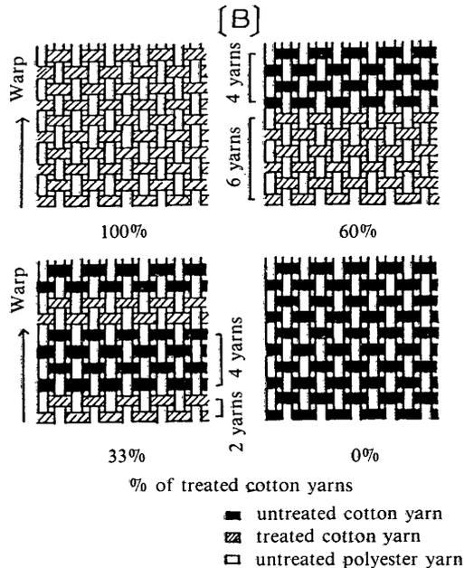
Fig. 1 (B) Diagram of the ratio of treated/untreated cotton yarn.
