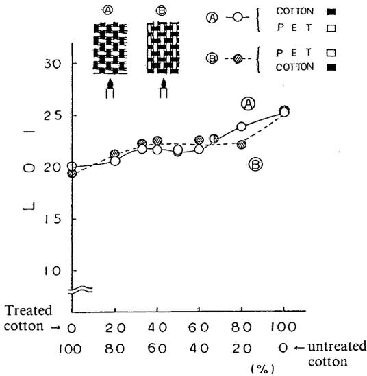
Fig. 5 Effect of the ratio of the THPC treated cotton yarn and the untreated one on the limiting oxygen index for the union cloth (cotton: PET = 0.5:0.5) A direction (—○—), B direction (---●---)
