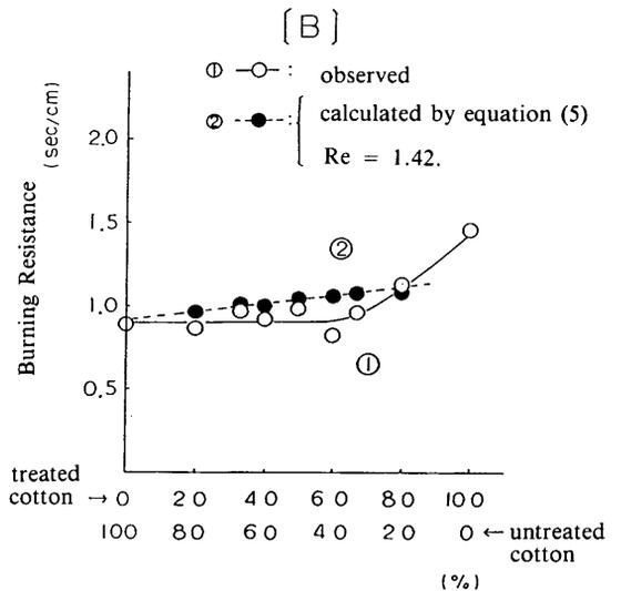
Fig. 4 (B) Observed (—○—) and calculated (---●---) burning resistance for the union cloth (Treated cotton yarn and untreated one: untreated polyester yarn = 50:50)
