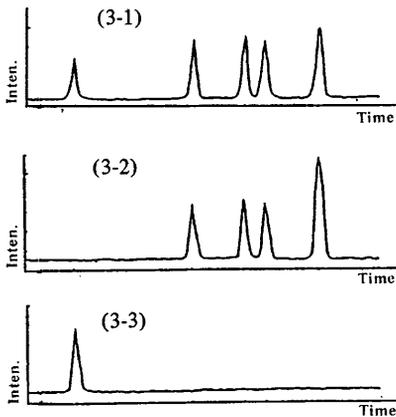
Figs. 3-1, 3-2, 3-3 Chromatograms of alkaline, acidic hydrolyzed proteins, and  $\gamma$ -carboxyglutamate
